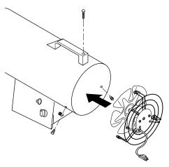
Figure 16 - Replacing Motor and Fan Guard into Heater
